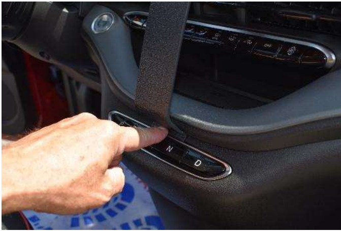
(5) Press the lower edge all the way into the lower seam. The tape will not leave any residue if the mount is removed in the future.
