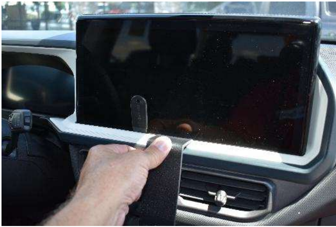
(5) Flex the top edge of the mount up and hook the thin top edge into the top seam.
