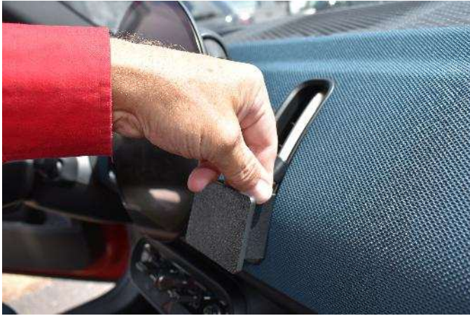
(5) Flex the m out and then press the thin edge into the other seam on the vent.
