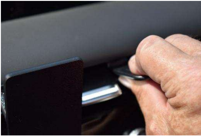
(5) Use the seam tool to open the upper seam a little.
