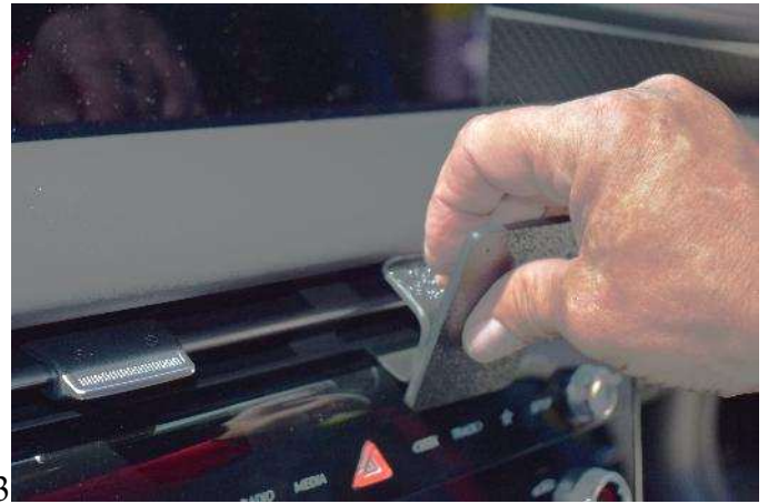
3 (6) Flex the top edge of the mount down and press the thin upper edge of the mount into the upper seam. The tape will not leave any residue if the mount is removed in the future.
