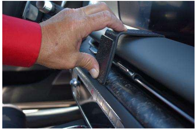
(6) Flex the mount down and insert the lower edge of the mount all the way into the lower seam.
