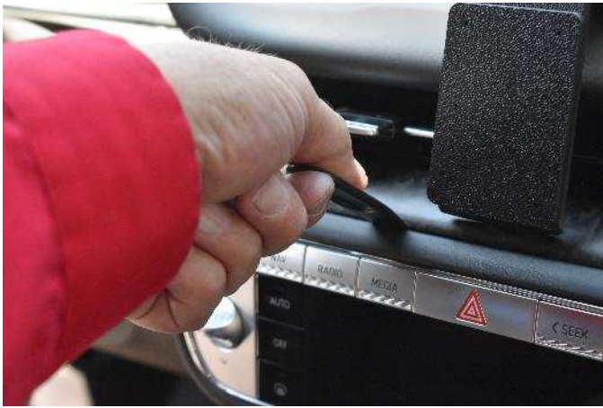
(5) Use the seam tool if needed to open the lower seam a little.
