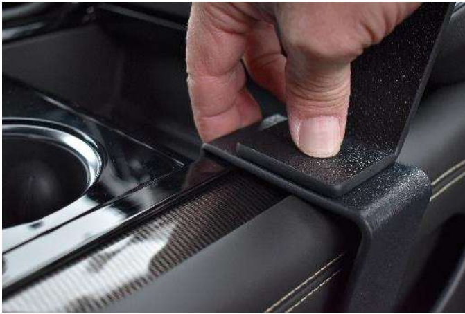
(5) Flex the mount to the left and hook the left edge of the mount onto the right panel edge.
