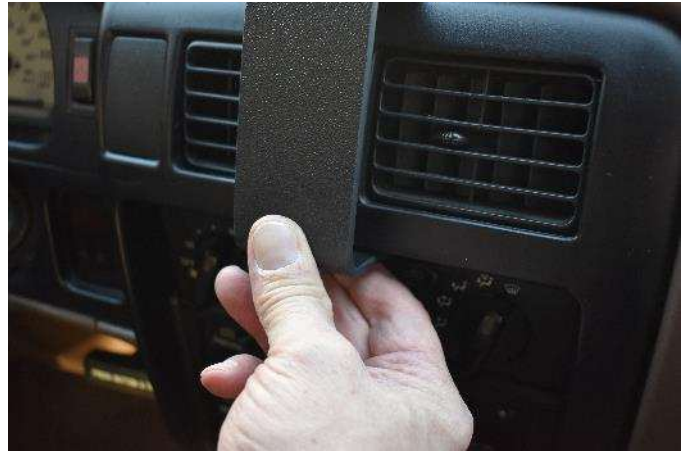
(6) Press the lower notched edge into the seam until the notch hooks onto the lower panel. The tape will not leave any residue if the mount is removed in the future.
