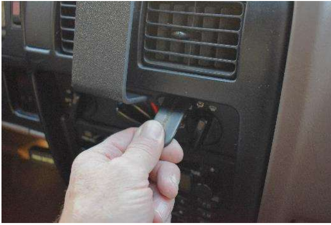
(5) Use the seam tool to open the lower seam a little.
