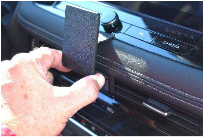
(5) Flex the lower edge of the mount down and into the lower seam.
