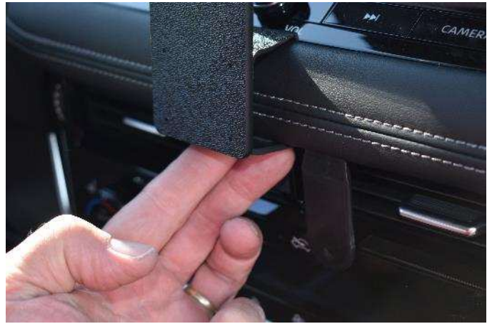
(6) Press the edge of the mount all the way into the seam.
