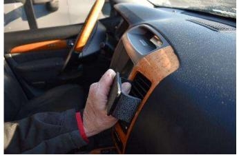
(2) Press the thin left edge of the mount into the seam right behind the left vent frame. When in the seam, the mount will not affect the vent louvers. Use the seam tool if needed to open the seam a little
