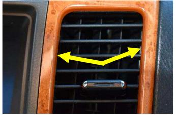
(1) Clean the area where the mount will attach. The right and left edges of the mount will attach right behind the frame around the center vents illustrated with the arrows in the photo above. Remove the covering from the tape.
