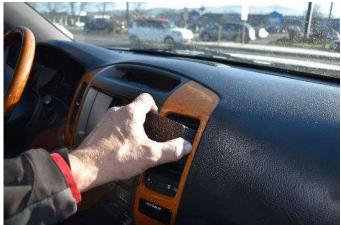
(3) Flex the right side of the mount inward and then press the right mount edge into the right seam behind the vent frame.
