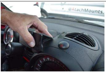
(4) Insert the thin front edge of the mount into the seam next to the seam tool.
