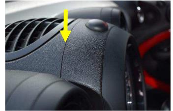
(1) Clean the area where the mount will attach. The upper edge of the mount will attach into the seam between the two trim panels around the display illustrated with the arrow in the photo above.
