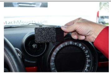
(5) Flex the lower edge of the mount towards you and hook the edge of the mount onto the frame around the speedometer.
