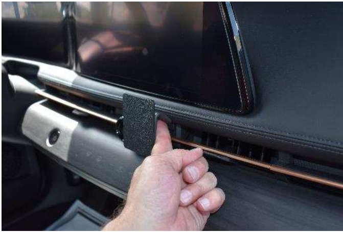
(5) Press the mount edges all the way into the seams.
