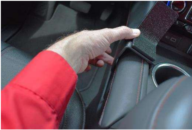
(5) Flex the left edge of the mount down and hook the lower edge under the side of the center console panel.
