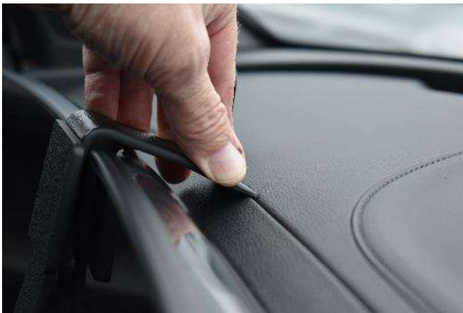
(5) Press the thin top edge of the mount into the top seam.
