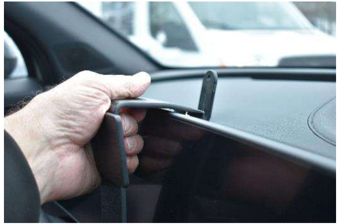
(6) Flex the top of the mount up and over the display.
