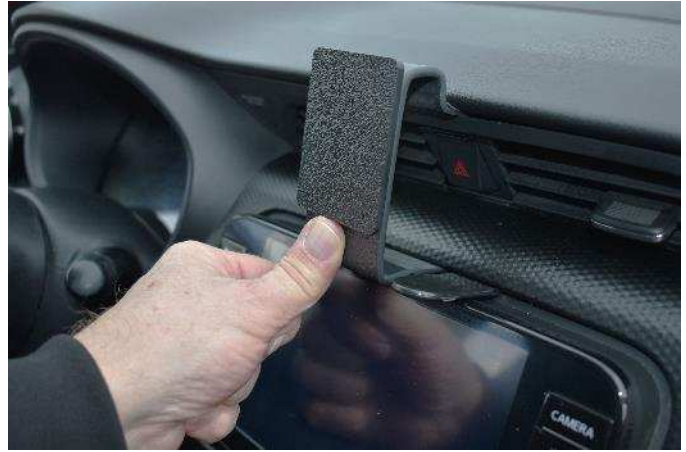
(6) Press the thin lower edge of the mount into the lower seam until the notch on the bottom of the mount clips onto the top of the display frame. The tape will not leave any residue if the mount is removed in the future.
