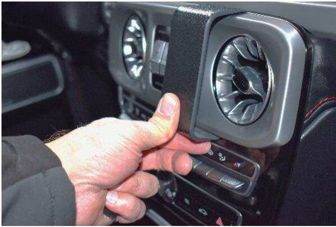
(5) Press forward on the lower edge to hook the lower edge of the mount into the lower seam.
