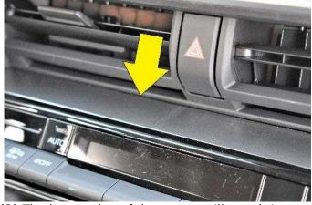
(2) The lower edge of the mount will attach into the seam under the center vents illustrated with the arrow in the photo above.
