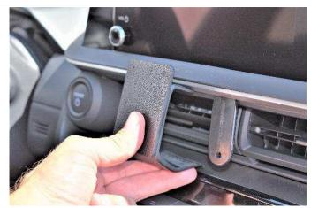
(5) Flex the lower edge of the mount up and forward to insert the lower edge into the lower seam. Press both the top and bottom edges all the way into the seams so the tape touches the panels.
