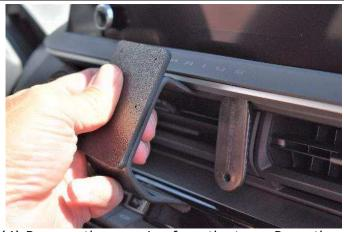
(4) Remove the covering from the tape. Press the thin top edge of the mount into the upper seam.
