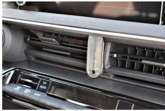
(3) Use the seam tool if needed to open the seam a little.
