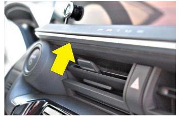
(1) Clean the area where the mount will attach. The upper edge of the mount will attach into the seam just behind the silver trim illustrated with the arrow in the photo above.
