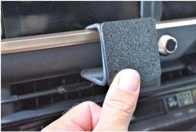
(5) Press forward on the lower edge of the mount until the thin lower edge goes into the lower seam.
