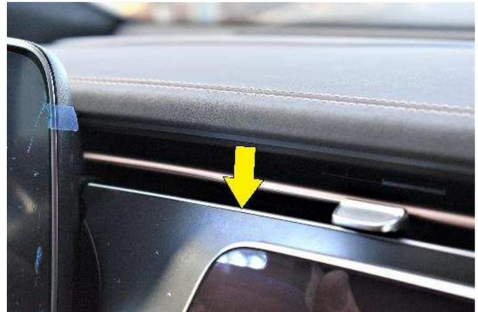
(2) The lower notched edge of the mount will rest on the lower vent frame.
