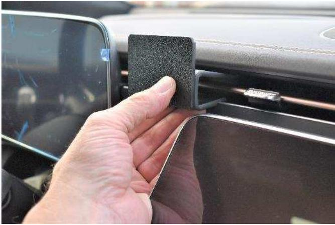
(5) Flex the lower edge of the mount up and hook the notched edge onto the lower vent frame.
