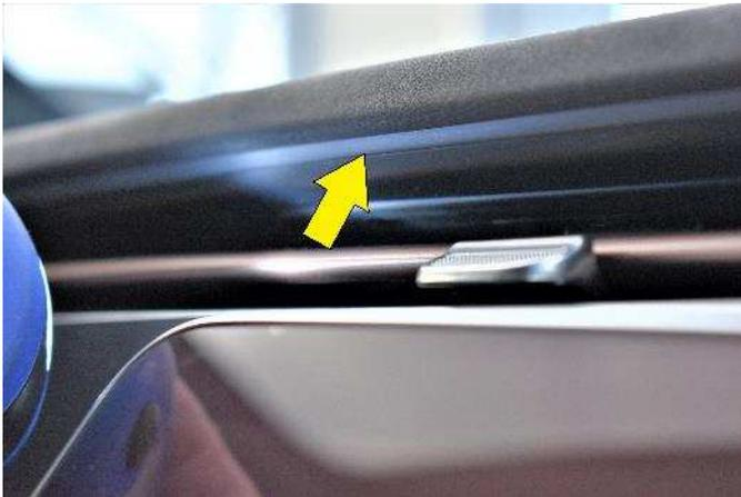
(1) Clean the area where the mount will attach. The top edge of the mount will attach into a seam that is difficult to see illustrated with the arrow above.
