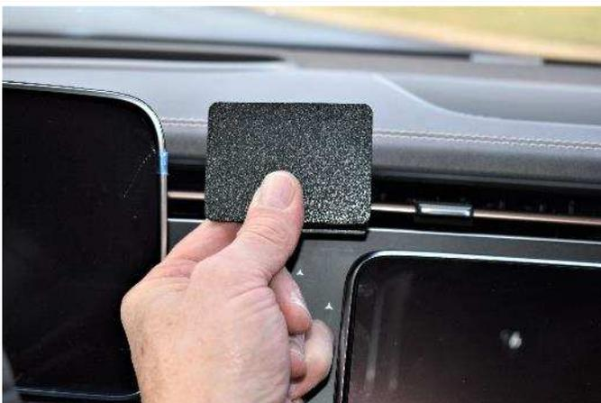
(3) Align the right edge of the mount with the top left edge of the display frame. This is the only place the mount will attach.
