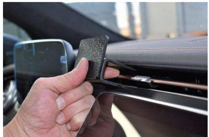
(4) Remove the covering from the tape. Press the thin top edge of the mount into the top seam.
