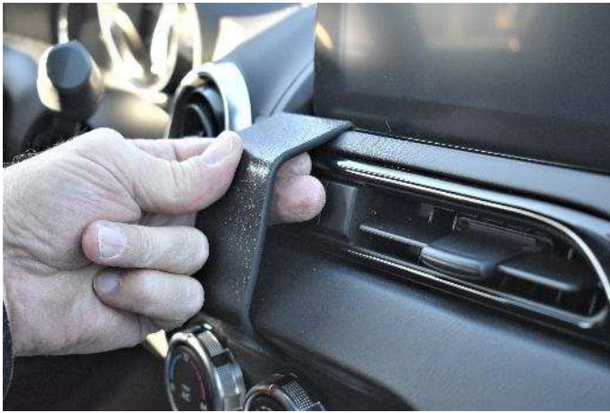
(5) Flex the top of the mount up and hook it onto the edge of the dash top.
