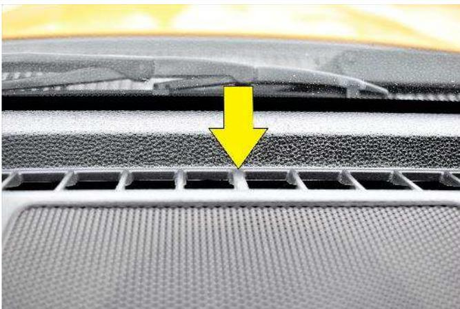
(1) Clean the area where the mount will attach. The front edge of the mount will attach into a seam in the defrost vent opening illustrated with the arrow in the photo.
