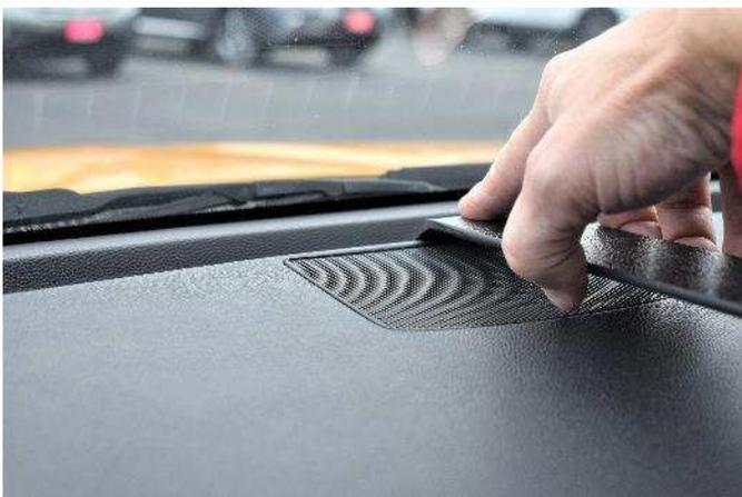
(3) Remove the covering from the tape. Hook the front edge of the mount into the front seam. The seam is right below the defrost grill panel.
