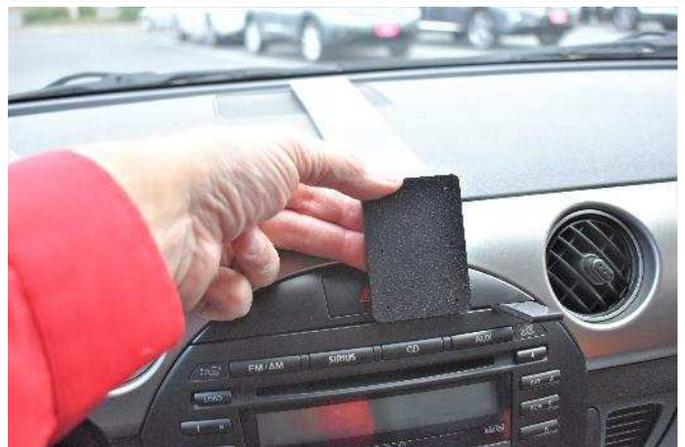
(4) Use the seam tool if needed to open the lower seam a little. Flex the mount out and press the lower edge into the lower seam. The tape will not leave any residue if the mount is removed.
