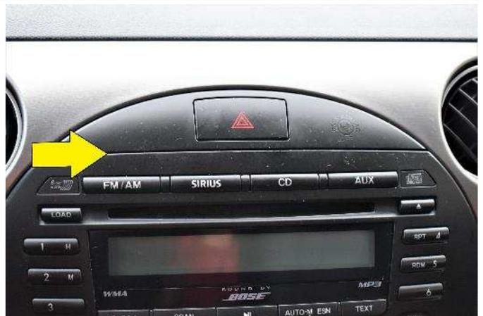
(2) The lower edge of the mount will attach into the seam illustrated in the photo above.
