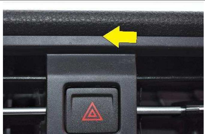
(2) The upper notched edge of the mount will attach into the seam illustrated with the arrow in the photo above.
