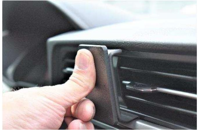
(6) Press the notched upper edge of the mount into the upper seam until the notched edge clips onto the frame around the vent. The tape will not leave any residue if the mount is removed in the future.
