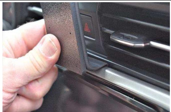
(4) Remove the covering from the tape. Press the thin lower edge of the mount into the lower seam.
