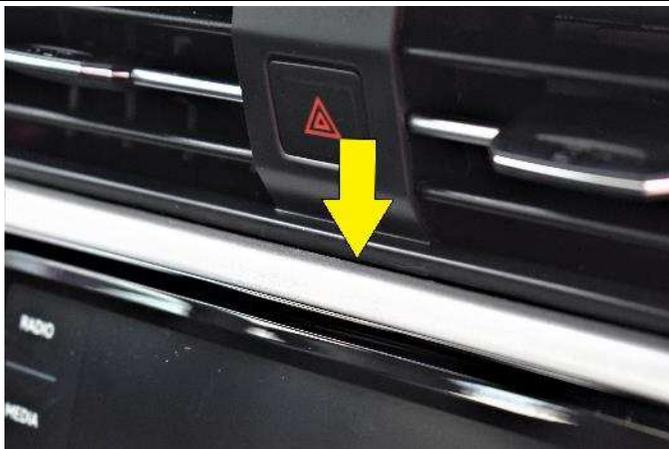
(1) Clean the area where the mount will attach. The lower edge of the mount will attach into the seam illustrated with the arrow in the photo above.
