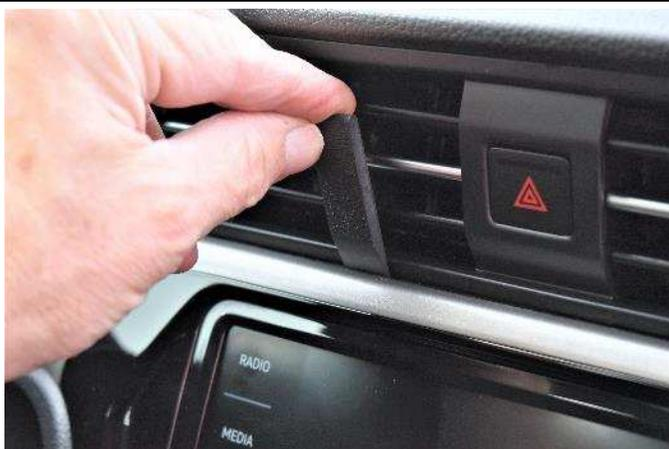
(3) Use the seam tool if needed to open the lower seam a little.
