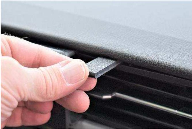
(5) Use the seam tool if needed to open the upper seam a little.
