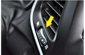
(1) Clean the area where the mount will attach. The top edge of the mount will attach into the seam just behind the lower vent fame illustrated with the arrow in the photo above.
