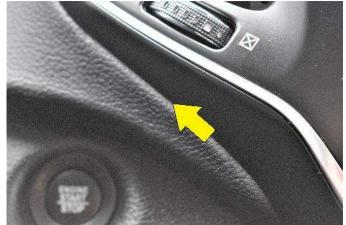
(2) The lower edge of the mount will attach into the seam illustrated with the arrow in the photo above.
