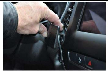
(5) Press down on the Mount to flex the lower edge into the lower seam.
