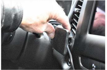
(4) Hook the top edge of the mount onto the lower vent frame and press the thin edge of the mount into the unseen seam right behind the frame.
