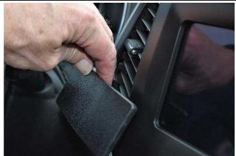
(6) Press down on the top edge to make sure the mount goes into the seam and the tape connects. The tape will not leave any residue if the mount is removed in the future.
