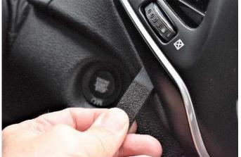
(3) Use the seam tool to open the lower seam a little. Remove the covering from the tape on the mount.
