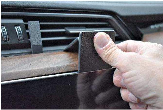
(5) Press the Mount forward to flex the front edge into the front seam.
