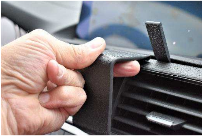
(5) Lift the top of the mount up and flex it into the upper seam.
