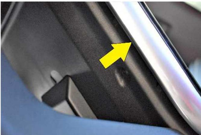
(1) Clean the area where the mount will attach. The notched top edge of the mount will attach onto the underside of the silver trim panel on the right or left side of the center console illustrated with the arrows in the photo above.
