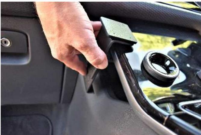
(3) Remove the covering from the tape. Hook the notched top edge of the mount under the panel illustrated in the photo above.
