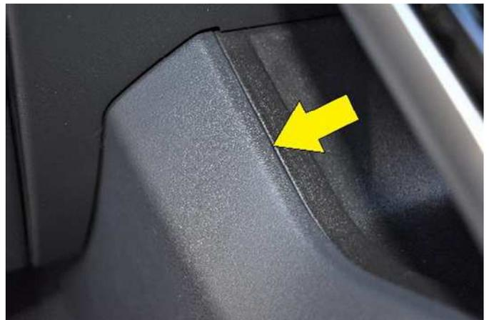
(2) The thin lower edge of the mount will attach into the seam illustrated with the arrows in the photo above. Use the seam tool if needed to open the seam a little. The tape will not leave any residue if the mount is removed in the future.
