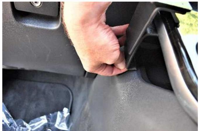
(4) Flex the lower edge of the mount up and into the lower seam. The mount needs to fit tight so it will take some pressure to flex into place.
