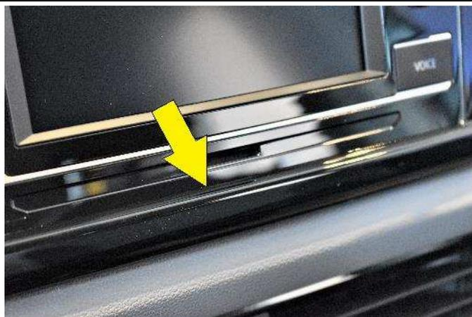
(1) Clean the area where the mount will attach. The upper edge of the mount will attach into the seam between the frame around the display and the dash panel covering the display illustrated with the arrows in the photo.
