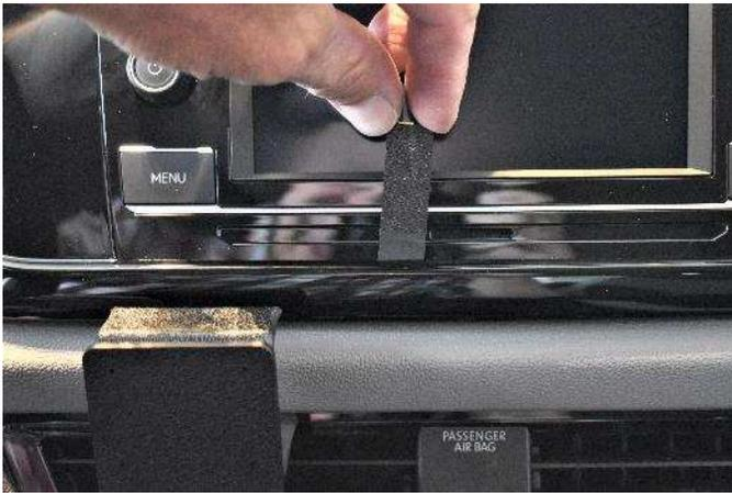
(5) Remove the seam tool and insert it into the seam illustrated in photo 1.
