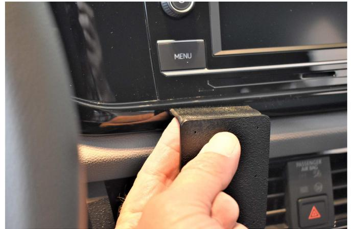
(6) Using two hands lift the upper edge of the mount up and forward into the upper seam. The tape will not leave any residue if the mount is removed in the future.
