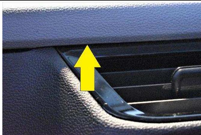
(2) The lower edge of the mount will attach into the seam between the frame around the vents and the separating dash panel above the vents illustrated with the arrows in the photo.
