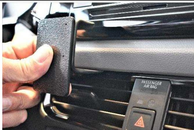
(4) Remove the covering from the tape. Then press the thin lower edge of the mount into the lower seam. The lower side of the mount is longer.
