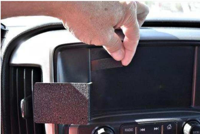
(5) Use the seam tool if needed to open the right seam a little.
