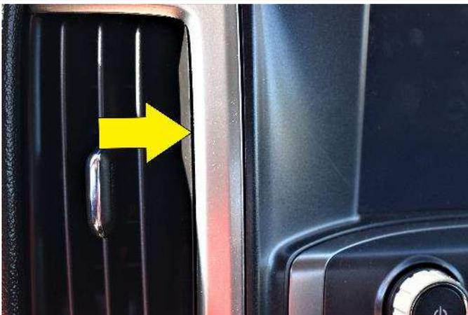
(1) Clean the area where the mount will attach. The left edge of the mount will attach into the seam illustrated with the arrow in the photo.
