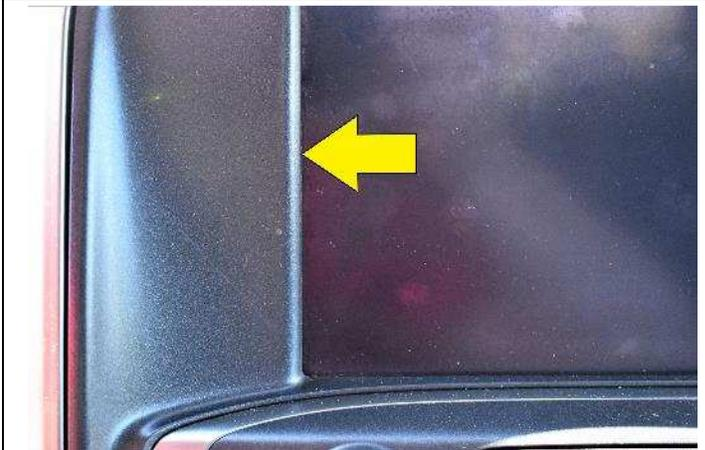
(2) The right edge of the mount will attach into the seam illustrated with the arrow in the photo.
