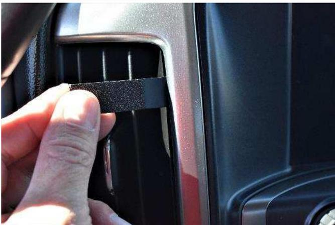
(3) Use the seam tool if needed to open the left seam a little.
