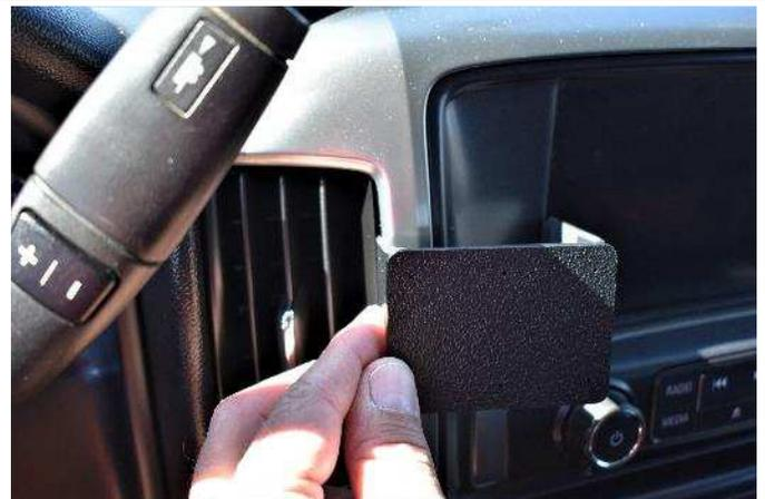
(4) Remove the covering from the tape. Insert the thin left edge of the mount into the seam.
