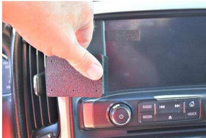
(6) Press the right side of the mount forward and hook the thin right edge of the mount into the seam. The tape will not leave any residue if the mount is removed in the future.
