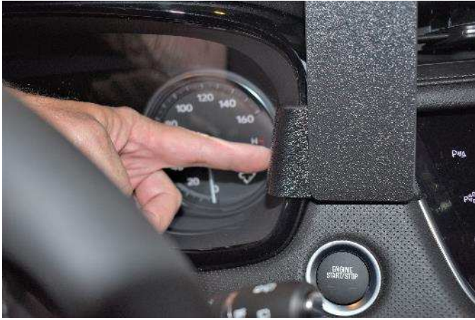
(5) Press inward on the edges to make sure the tape connects with the panels.
