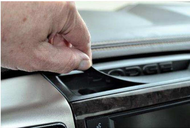
(1) Clean the area where the mount will attach. Remove the rubber pad from the bottom of the dash top tray.
