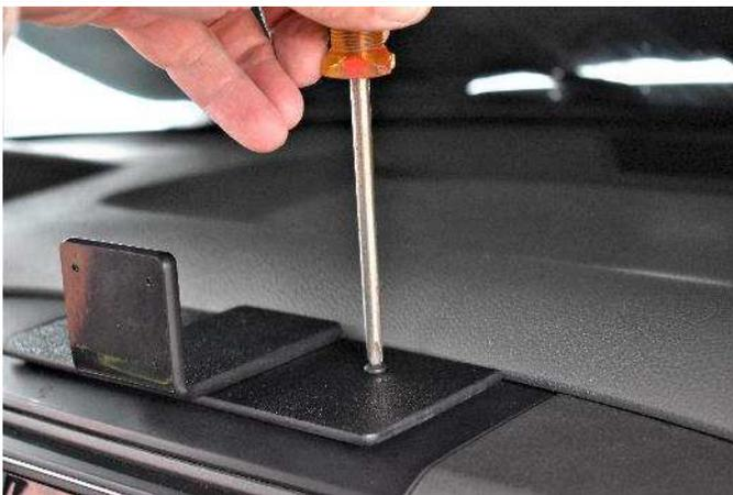
(3) Use the outside holes for the 2009 - 2012 models and the inside holes for the 2013 - 2018 models. Using the included screws insert the screws into the correct holes and tighten into the holes where the original screws were removed from.
