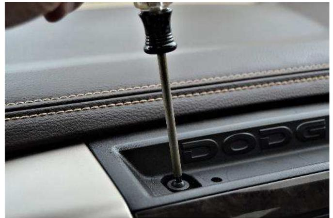
(2) Remove the two screws that hold the dash top tray down.
