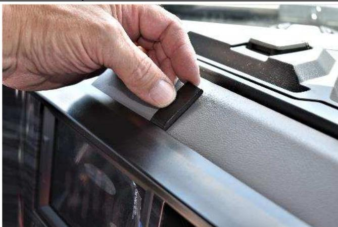
(3) Insert the thin edge of the seam tool into the front seam to open the seam a little.
