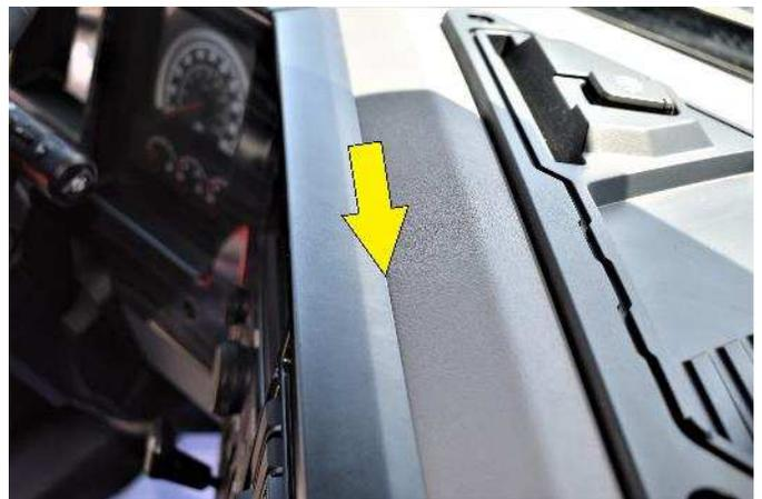
(2) The upper / forward edge of the mount will attach into the seam illustrated with the arrow in the photo.
