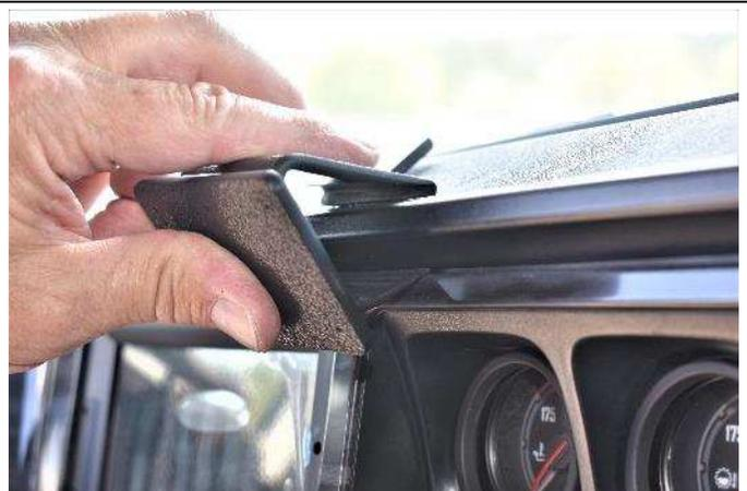
(4) Remove the covering from the tape. Hook the lower edge of the mount under the dash top and into the opening illustrated in photo one.
