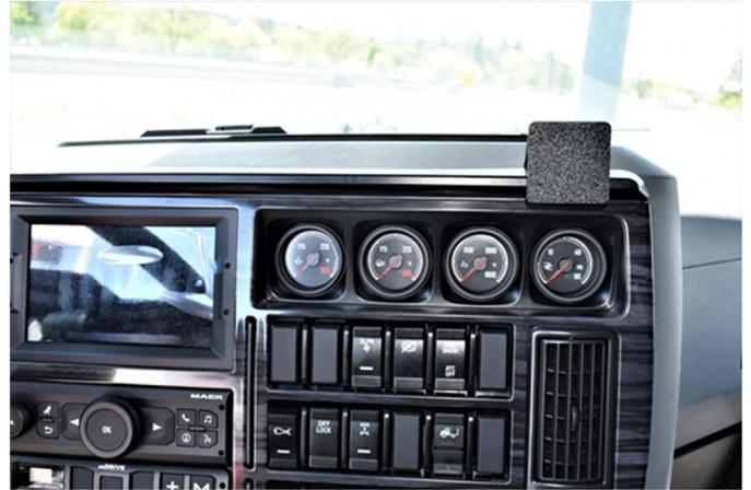
(6) The mount attached. The tape will not leave any residue if the mount is removed in the future.
