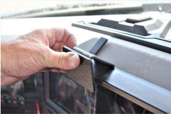
(5) Press forward on the top of the mount until the thin front edge hooks into the front seam.
