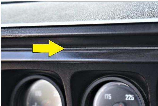
(1) Clean the area where the mount will attach. The lower edge of the mount will attach into the opening below the dash top illustrated with the arrow in the photo.
