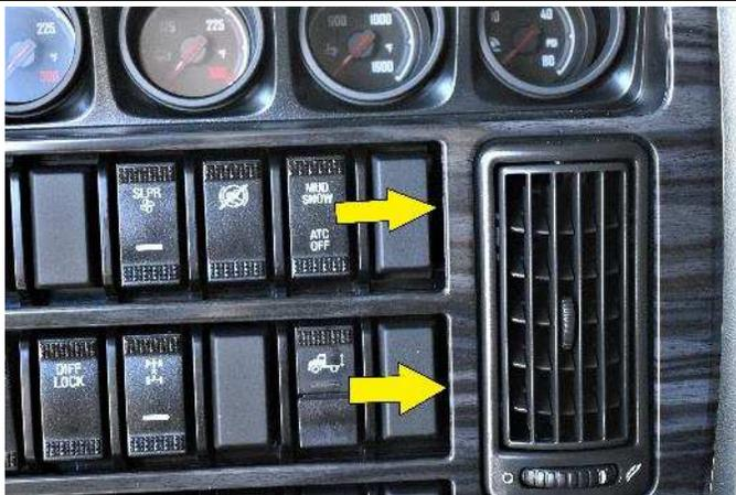
(1) Clean the area where the mount will attach. The left edge of the mount will attach into either of the two seams illustrated with the arrows in the photo.
