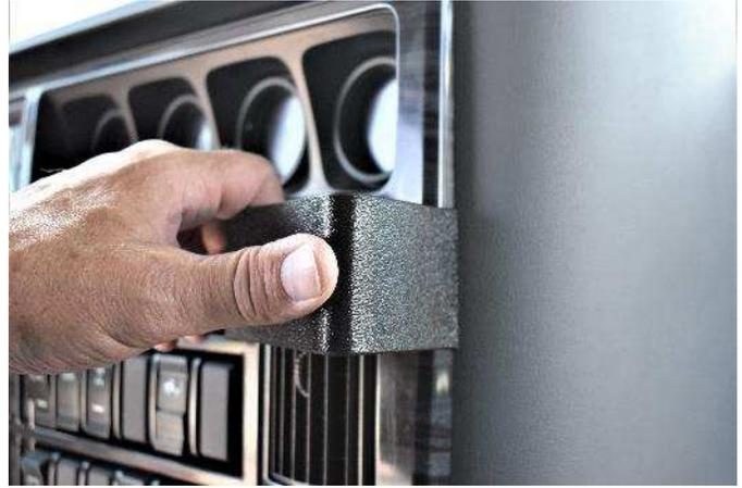
(6) Press the right side of the mount forward until the right edge of the mount hooks onto the right side of the dash panel. The tape will not leave any residue if the mount is removed in the future.
