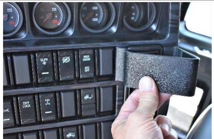
(4) Remove the covering from the tape. Hook the thin left "J" shaped edge onto the dash panel to the left of the vent frame. See photos.
