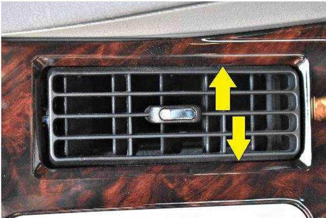
(1) Clean the area where the mount will attach. The mount will attach into two seams that are right behind the top and bottom frame around the vents illustrated with the arrows in the photo.
