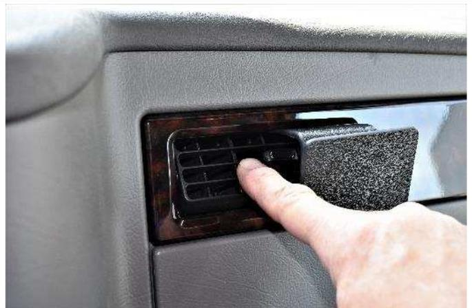
(4) Tilt the vent louvers upward to gain access to the top seam.
