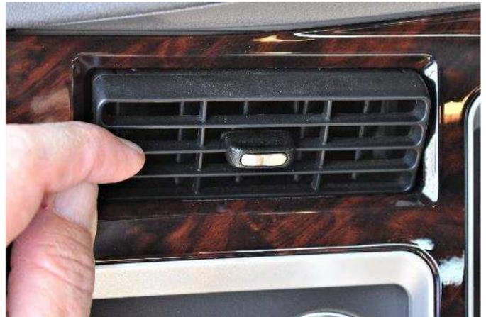
(2) Tilt the vent louvers down to gain access to the lower seam. Remove the covering from the tape on the mount.
