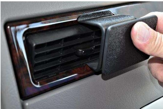
(3) Hook the thin lower edge of the mount over the vent frame and into the seam behind the frame.
