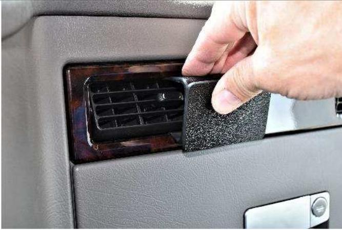
(5) Flex the top of the mount down and hook the top edge of the mount onto the top frame of the vent and into the top seam.
