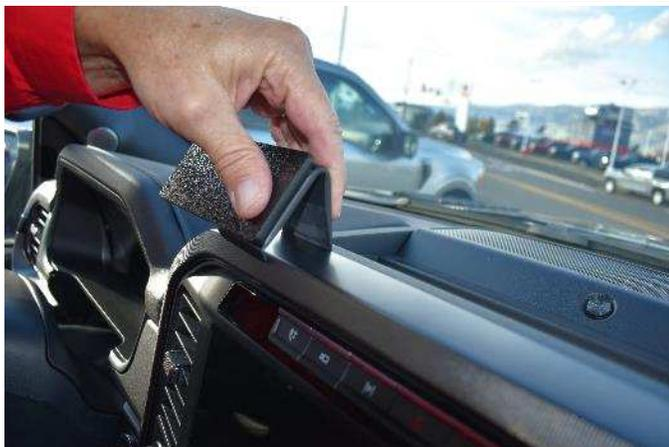
(3) Press the thin front edge of the mount into the seam illustrated in the photo above. Use the seam tool to open the seam a little if needed.
