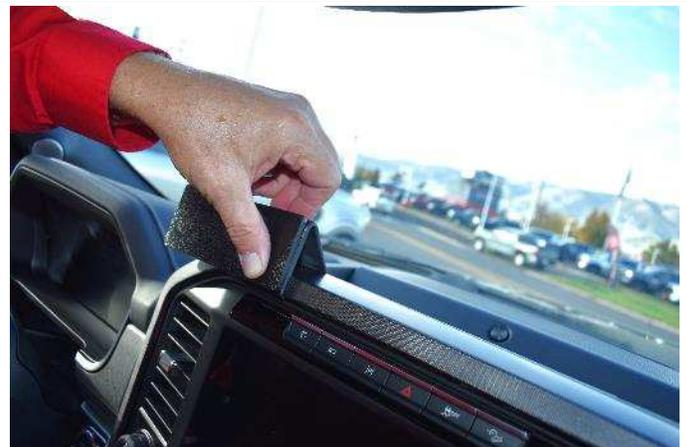
(4) Press down and forward on the faceplate to hook the lower edge under the dash top frame. The tape will not leave any residue if the mount is removed in the future.
