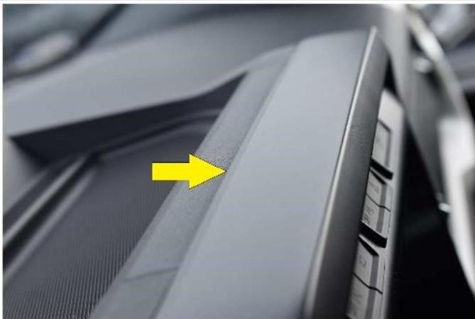
(1) Clean the area where the mount will attach. The front edge of the mount will attach into the seam in front of the top display frame illustrated with the arrow in the photo.
