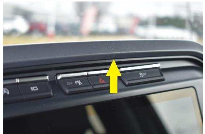
(2) The lower edge of the mount will attach onto the top display frame illustrated with the arrow in the photo. **Remove the covering from the tape.**
