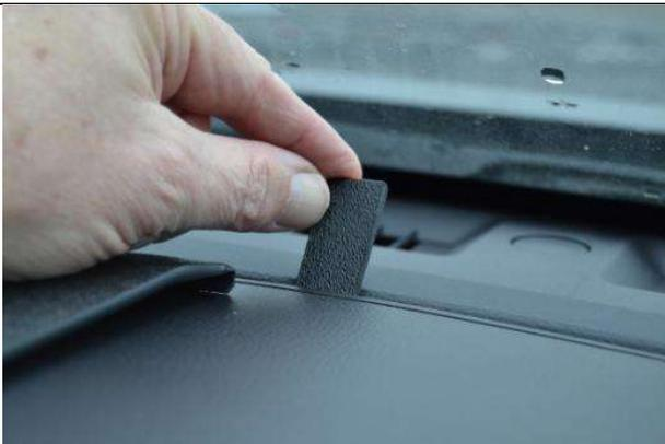
(3) Insert the seam tool into the seam between the padded dash top and the frame around the defrost vent near the windshield. See photo. The tape will not leave any residue if the mount is removed in the future.
