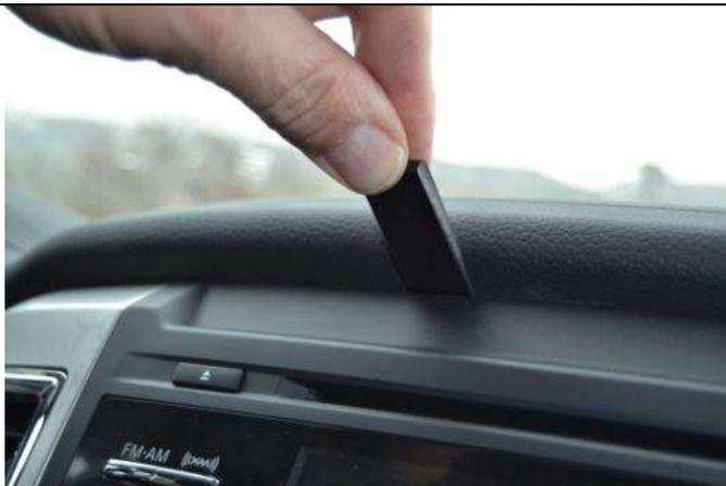
(1) Clean the area where the mount will attach. Remove the covering from the tape. Insert the seam tool into the seam between the padded dash top and the top of the frame around the radio.
