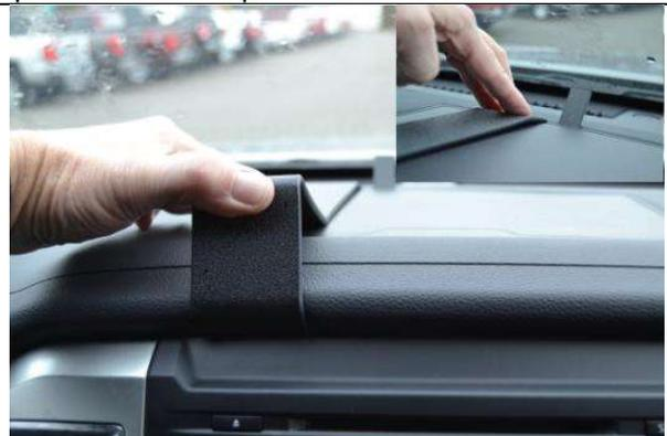
(4) Press forward on the top of the face plate of the mount to flex the front of the mount into the seam next to the seam tool. Press firmly down on the front edge of the mount so the mount edge goes all the way into the seam.
