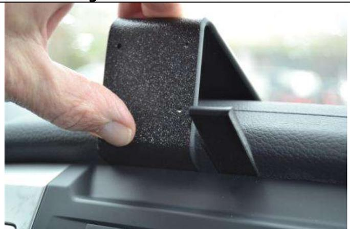
(2) This might be a tight seam and might take some pressure to open the seam. Press the lower edge of the mount all the way into the seam until the back of the mount face plate bumps against the padded dash top. Remove the seam tool.
