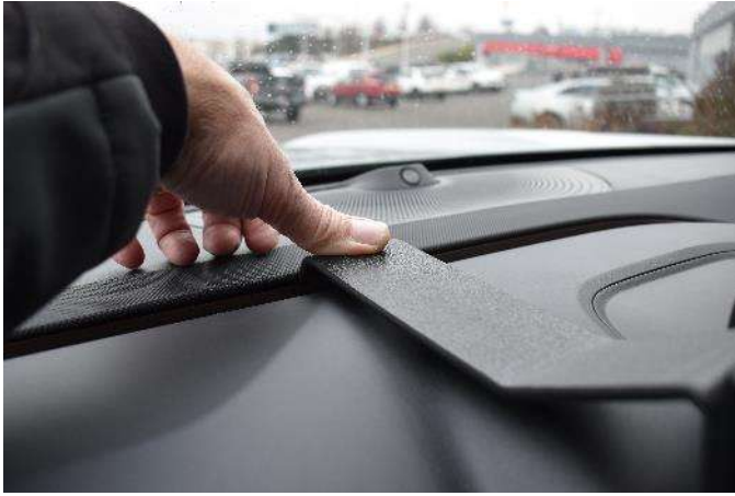
(5) Press the notched edge of the mount all the way into the front seam until the mount slips into place.
