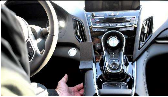
(5) Press upward on the Mount to make sure the mount edge goes all the way into the lower seam.
