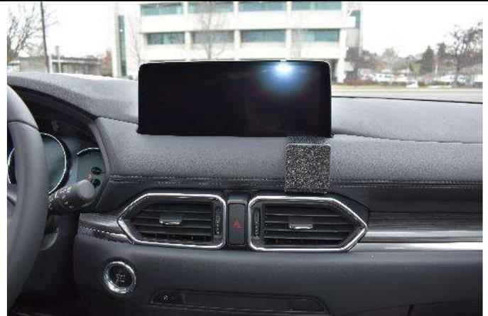
(4) The mount attached. The mount will attach over the entire center vent area above the vents. The tape will not leave any residue if the mount is removed in the future.
