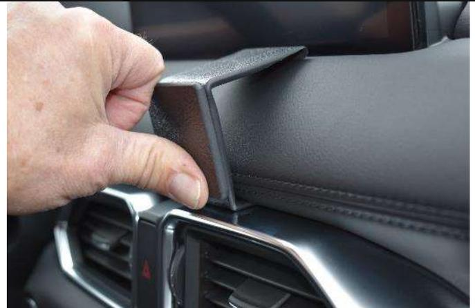
(2) Press the bottom of the mount into the lower seam until the back of the mount bumps onto the dash.
