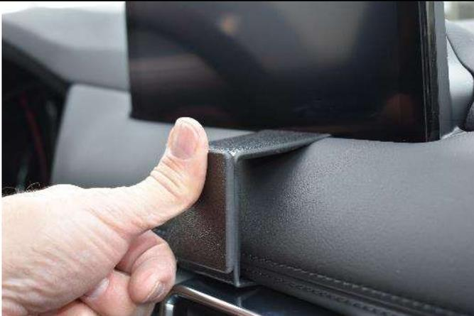
(3) Then press the top of the mount forward until the upper edge goes into the gap between display screen and the dash panel in front of the screen.
