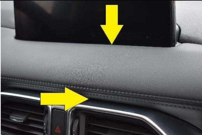
(1) Clean the area where the mount will attach. Remove the covering from the tape. The thin edges of the mount will attach into the two seams illustrated with the arrows in the photo above.
