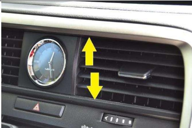
(1) Clean the area where the mount will attach. The mount will attach into a seam just behind the top vent frame and onto the lower vent frame illustrated with the arrows in the photo.
