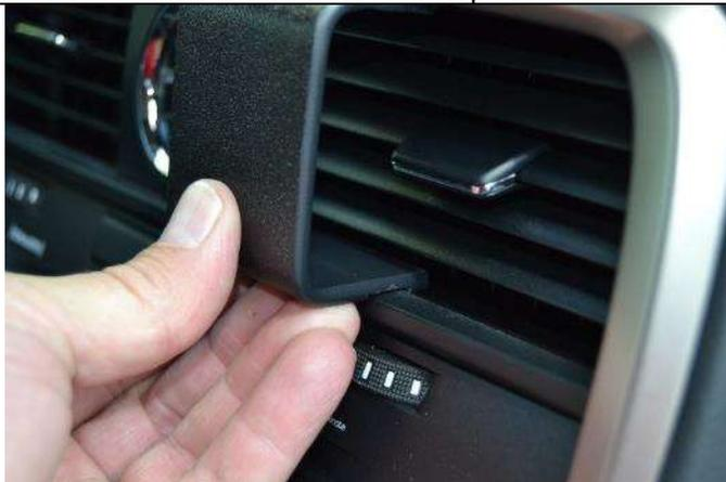
(3) Press up on the bottom of the mount and hook the lower notched edge of the mount onto the lower vent frame.
