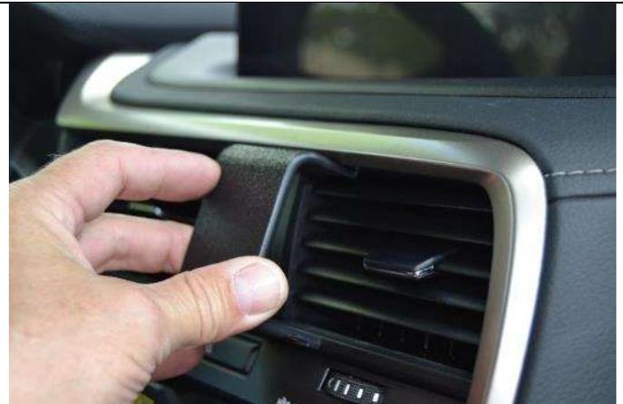
(2) Remove the covering from the tape. Insert the thin top edge of the mount into a seam right behind the top vent frame. You can feel the seam with your finger. The mount will fit into the seam.
