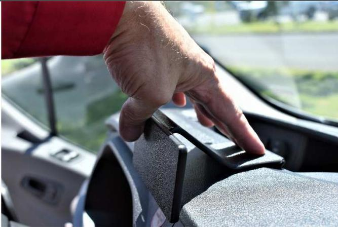
(5) Press forward on the top of the mount and, at the same time, press down on the front of the mount to hook the front "J" shaped edge of the mount into the front seam. Use the seam tool if needed to open the seam a little. Using two hands will help.
