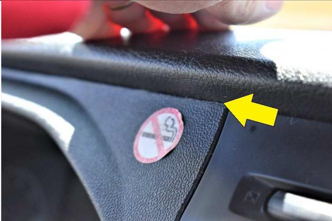
(1) Clean the area where the mount will attach. The thin lower edge of the mount will attach into the seam illustrated with the arrow in the photo above.
