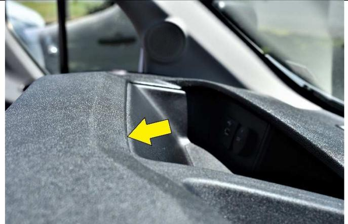
(2) The front "J" shaped edge of the mount will attach into the seam illustrated with the arrow in the photo above.
