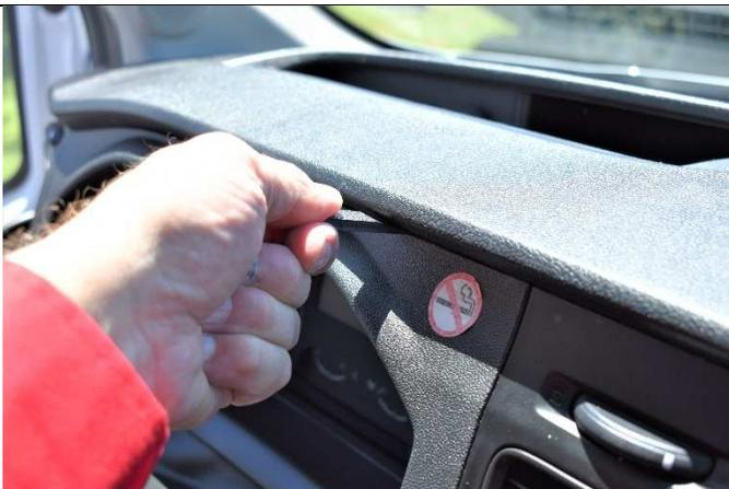
(3) Use the seam tool to open the lower seam a little for the mount to insert into. The right edge of the mount should align with the right edge of the lower panel.
