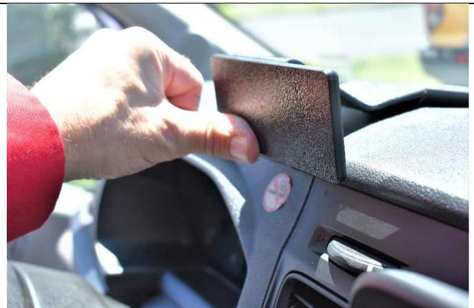
(4) Remove the covering from the tape. Press the thin lower edge of the mount all the way into the seam until the tape touches the dash top.
