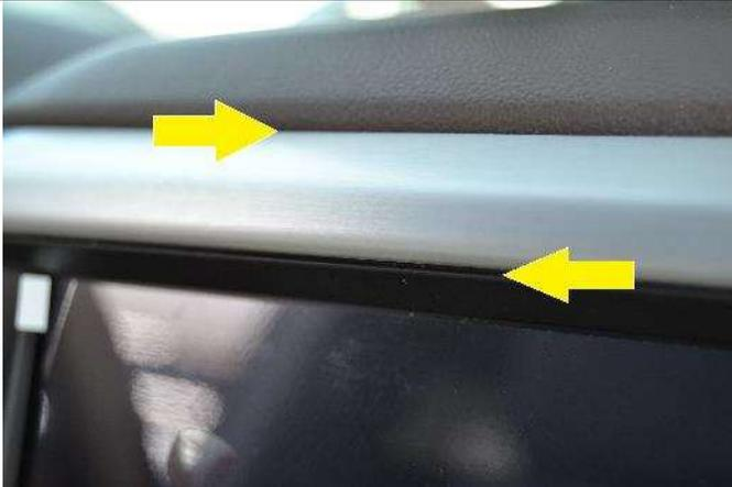
(1) Clean the area where the mount will attach. The mount will attach into the two seams illustrated with the arrows in the photo.
