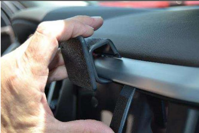
(3) Remove the covering from the tape. Position the mount in the location that best fits your needs. Insert the thin lower edge of the mount into the seam next to the seam tool. The tape will not leave any residue when the mount is removed.
