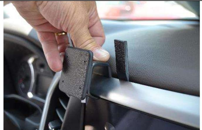
(4) Press the seam tool into the front seam next to the padded dash top to open the seam. Flex the front notched edge of the mount forward and downward into the front seam.
