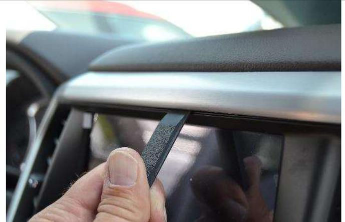
(2) Insert the thin edge of the seam tool into the seam between the frame around the display and the frame around the upper center console to open the seam.
