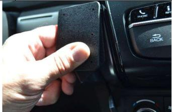
(4) Continue to press the left edge of the mount into the left seam as you rotate the mount to the right and into the right seam.
