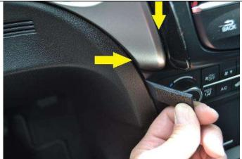
(1) Clean the area where the mount will attach. The mount will attach into the two seams illustrated with the arrows in the photo. Insert the seam tool into the left seam to open the seam a little.
