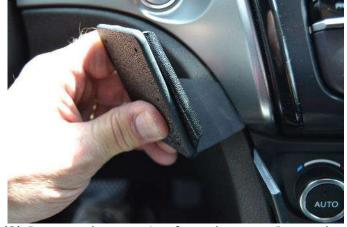
(2) Remove the covering from the tape. Insert the thin left edge of the mount into the seam. The mount edge should be at the bottom of the panel. See photo.
