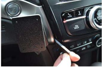
(3). Take the seam tool out and insert it into the right seam to open the seam a little.
