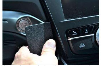
(5) Press down on the top of the mount to make sure the tape connects. The tape will not leave any residue if the mount is removed in the future.
