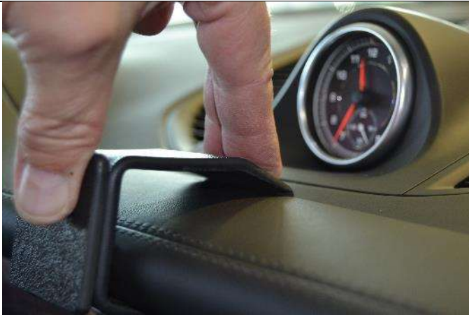
(5) Press the front of the mount all the way into the seam.
