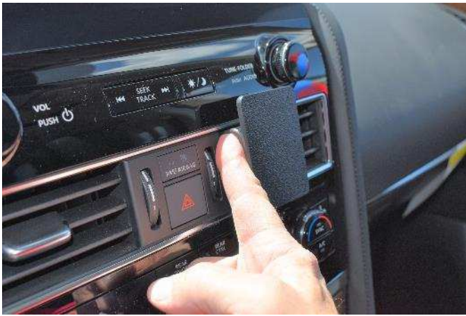
(5) Press the top and bottom edges all the way into the seams.
