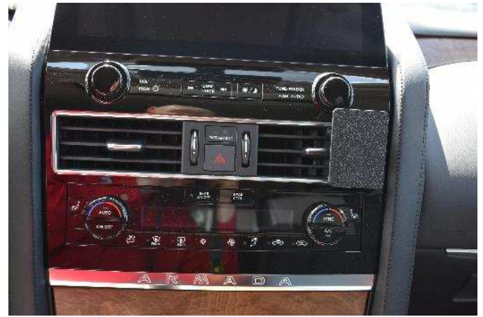
(6) The mount attached. The tape will not leave any residue if the mount is removed in the future.
