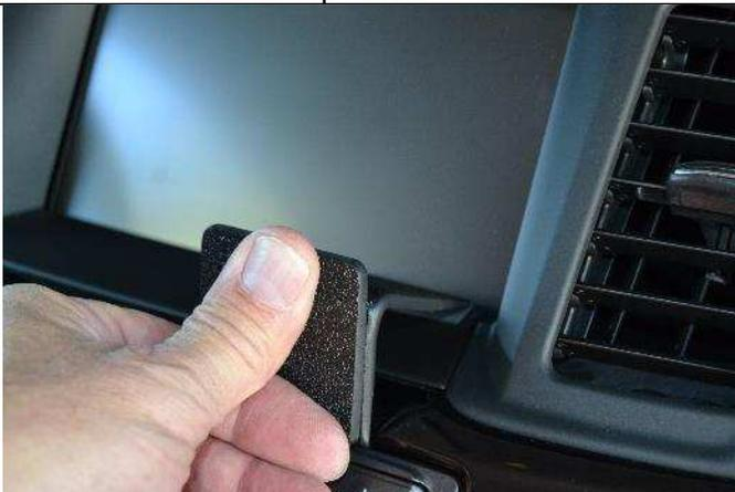
(3) Press forward on the face of the mount until the top/front edge of the mount goes into the seam between the display screen and the panel in front of the screen.
