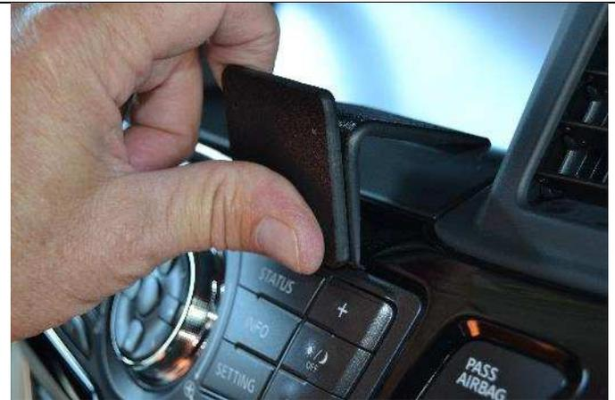
(2) Remove the covering from the tape. Press the bottom edge of the mount into the lower seam illustrated in the first photo.
