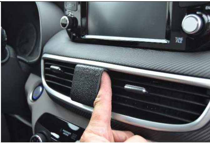
(5) Press the top and bottom of the mount into the seams to make sure the mount is securely attached.
