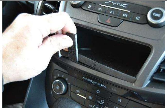
(2) Insert the thin edge of the seam tool into the seam behind the frame around the dash cubby. It is found under the rubber pad but the pad does not need to be removed.
