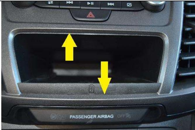
(1) Clean the area where the mount will attach. The mount will attach into the two seams just behind the top and bottom frame around the dash cubby illustrated with the arrows in the photo.
