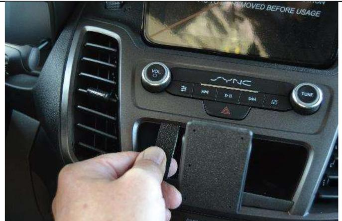
(4) Remove the seam tool and insert it into the top seam just behind the frame around the dash cubby.
