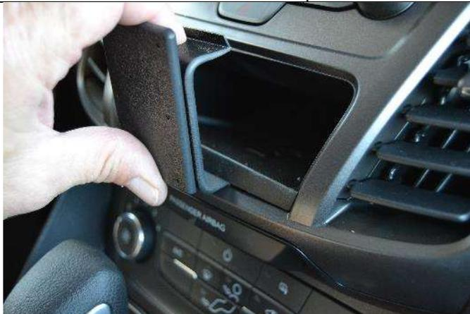
(3) Remove the covering from the tape. Insert the lower (Shorter) edge of the mount into the seam next to the seam tool. Starting with a corner of the mount will help to insert the edge.
