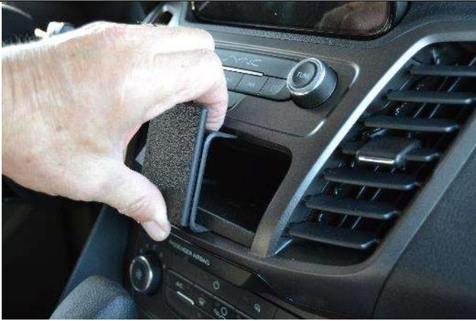
(5) Press the top of the Mount downward and insert the thin top edge of the mount into the top seam.
