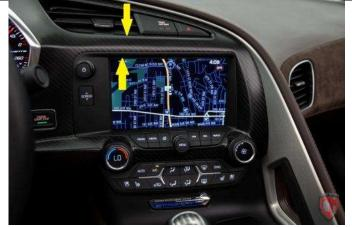
(1) Clean the area where the mount will attach. The bottom of the mount will attach under the far left upper frame around the center display and between the upper vent louver and frame in front of the vent. See arrows in the photo.
