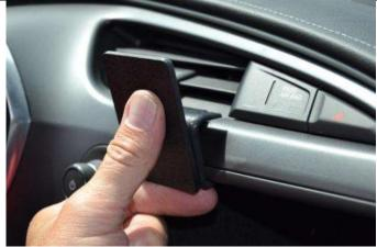
(3) Press the top of the mount forward until the upper edge goes into the seam between the upper vent louver and frame in front of the vent.
