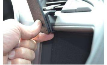
(2) Remove the covering from the tape. The tape will not leave any residue if the mount is removed in the future. Hook the lower edge of the mount under the far left upper frame around the center display.
