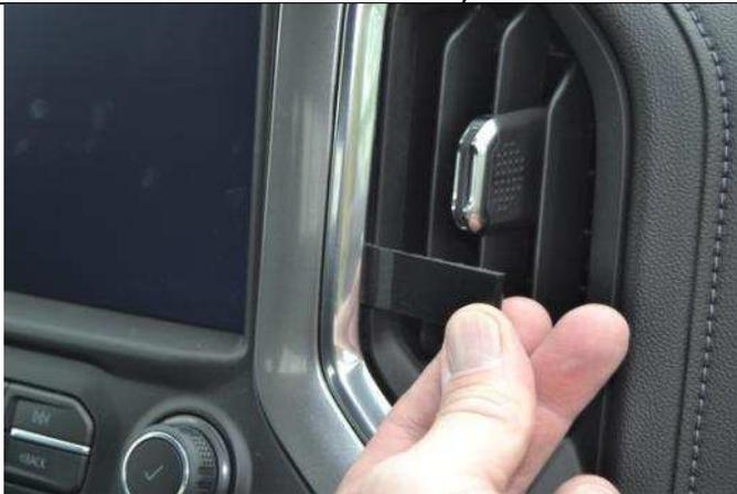
(1) Clean the area where the mount will attach. Insert the thin edge of the seam tool into the seam between the vent and the silver frame around the left side of the vent. The seam is very tight but it does open.
