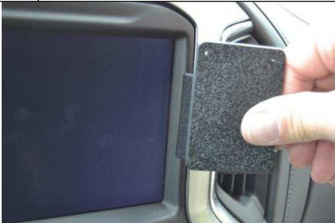
(3) Press the mount to the left to flex the thin left edge of the mount into the seam between the display screen and the right frame around the display.
