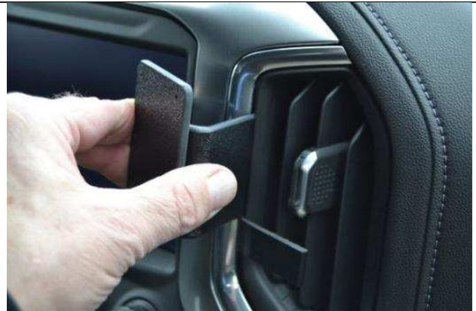
(2) Remove the covering from the tape. Insert the thin right edge of the mount into the seam next to the seam tool.
