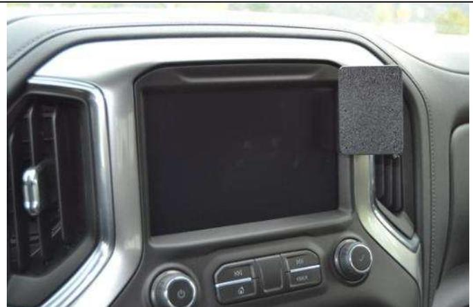
(4) The mount attached. The tape will not leave any residue if the mount is removed in the future. Remember to remove the seam tool from the seam.
