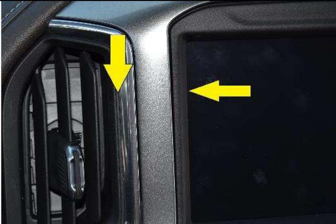
(1) Clean the area where the mount will attach. The two edges of the mount will go into the seams illustrated with the arrows in the photo.
