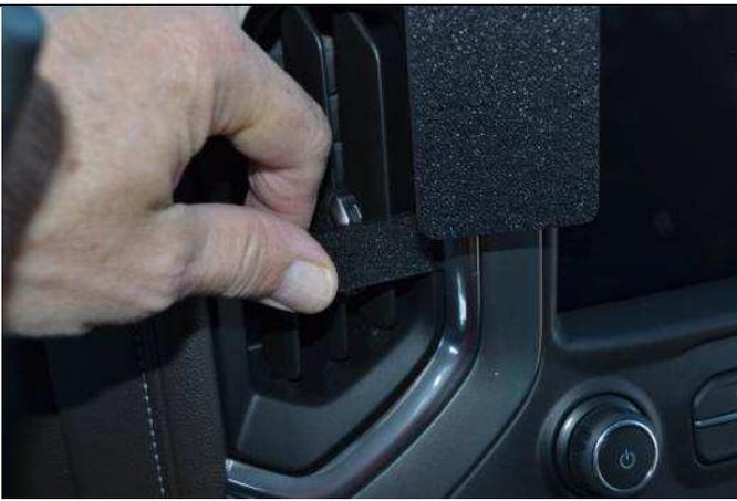
(5) You might need to press forward on the seam tool to open the seam a little for the mount to insert into the seam.
