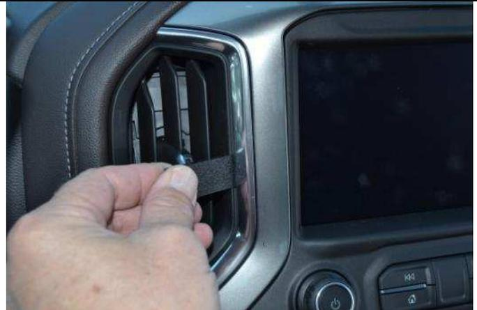
(2) Insert the thin edge of the seam tool into the seam between the vent and the silver frame around the right side of the vent. The seam is very tight but it does open.
