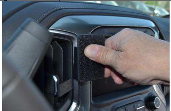
(4) Press the mount to the left to flex the thin left edge of the mount into the seam next to the seam tool.
