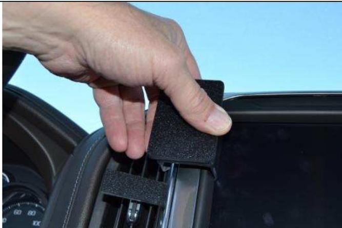
(3) Remove the covering from the tape. Insert the thin right edge of the mount into the seam between the display screen and the left display frame.
