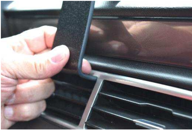
(5) Flex the lower edge of the mount down and hook the notched edge onto the top vent frame.
